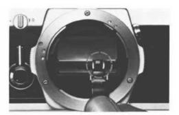
CAUTION: Although the above procedure can be done with fingers, it is recommended that you use the special tool supplied. Changing focusing screens is a procedure to be exercised with great care. Trying to change a screen with your fingers can result in fingerprints and costly damage to the surface of the screen, the prism, or the mirror. Should this occur, cleaning or repair MUST be handled by an authorized service center. Such damage is not covered by the product warranty.
