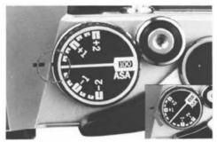
③ Once the setting has been made, turn the dial until the white line is aligned with the black index line on the pentaprism housing.
