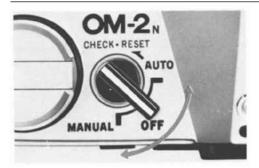
The selector lever on top of your camera has four positions as follows (with click stops at AUTO-OFF-MANUAL):
