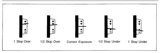
Manual exposure can be compensated by adjusting the F stop or shutter speed. The exposure needle indicates over-exposure at the (+) side, or under-exposure at the (-) side.
