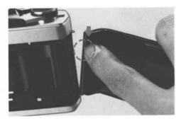
The camera back of the OM-2 is fully interchanbeable with the Recordata Back 2, 3 and 250 Film Back 1. To remove the camera back, push down on the release pin as shown. Do not remove the back unless necessary.
