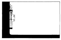
③ A red lamp lights in the viewfinder when the T32 (or T20) capacitor is charged ready for shooting. Set the aperture ring to the f/stop you require, focus on the subject and release the shutter. NOTE: All f/stops on the camera lens can be used.
