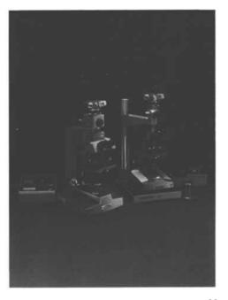
When the photographic magnification desired exceeds 10x, it becomes more difficult for the macrophotographic equipment alone to obtain excellent pictures. A sophisticated array of photomicrography accessories with a microscope as the central figure is required. The exciting vision of looking at the microscopic world through a microscope can be recorded by the OM-2.
