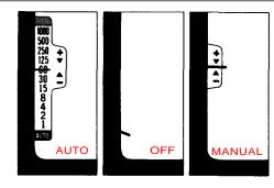
The three-position viewfinder control center allows you to see the operating mode of your camera without checking the position of the selector lever.
