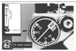
If you wish to change the exposure setting automatically selected by the camera, use the exposure compensation dial and a compensation marker appears in the viewfinder.
