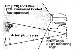
All required of the T32 (T20) is a flick of the on/off switch. The rest is taken care by the OM-2.
